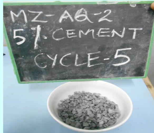
20mm size aggregate after soundness test, pre-coated with 5% cement.
