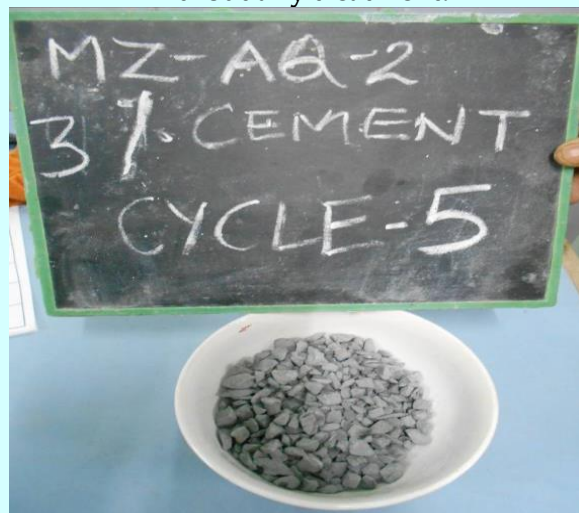
20mm size aggregate after soundness test, pre-coated with 3% cement.
