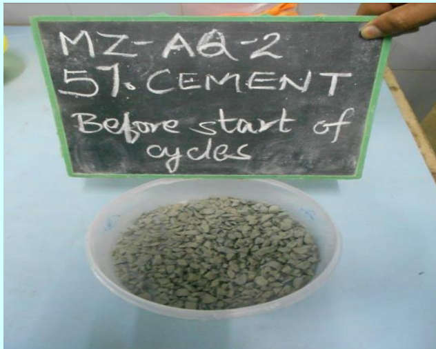
20mm size aggregate before the soundness test, pre-coated with 5% cement.
