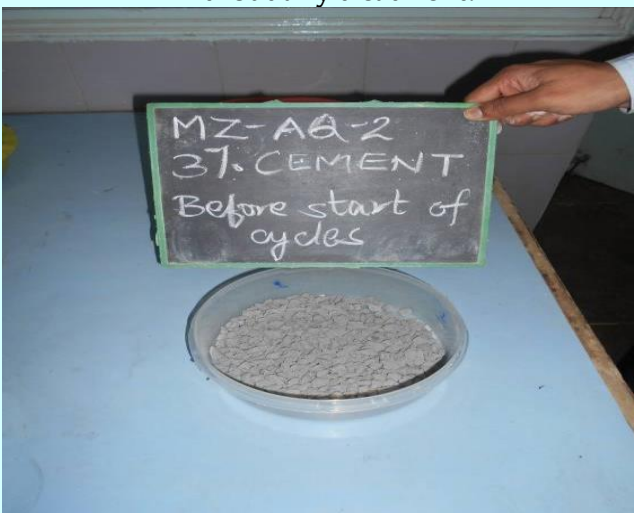
20mm size aggregate before the soundness test, pre-coated with 3% cement.
