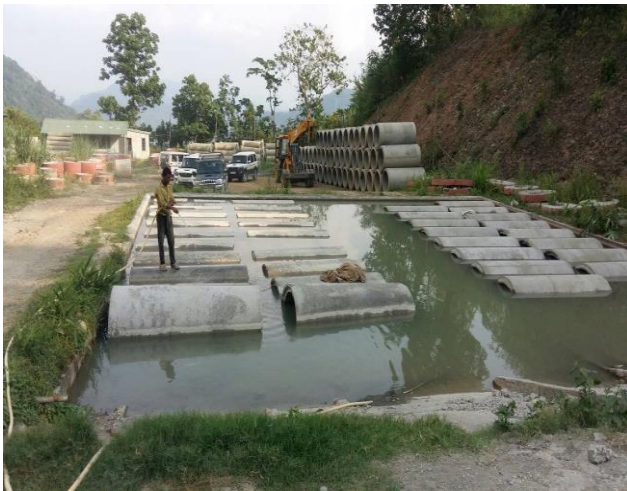
Manufacturing of Hume pipe at Contractor's Hume pipe factory
